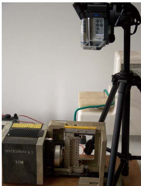
Figure 8. Experimentally stand for the study of motive electric operation with translational limited motion
